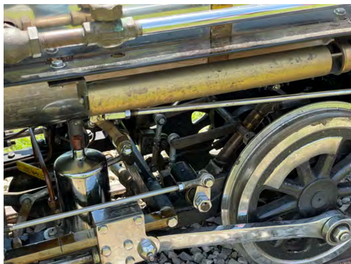
I was trying to get a shot of the Stevenson-style valve gear.
