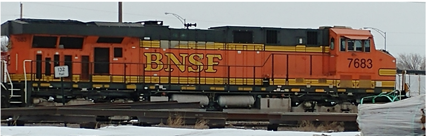
(Below) BNSF 7683 was built in March of 2005 as a GE ES44DC . The ES44DC series was produced between 2005 and 2010. The ES44DC (Evolution Series, 4,400 hp, DC traction motors) replaced the Dash 9-44CW model in the General Electric catalogue. Primary users are BNSF, CSX Transportation, and Canadian National Railway.
