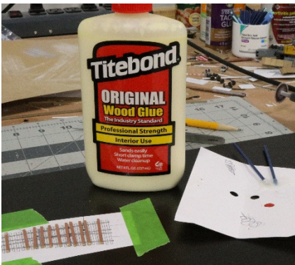
(left) We need to secure the PC ties to the paper template to prevent them shifting during construction, so we use regular carpenters glue to hold them in place.
