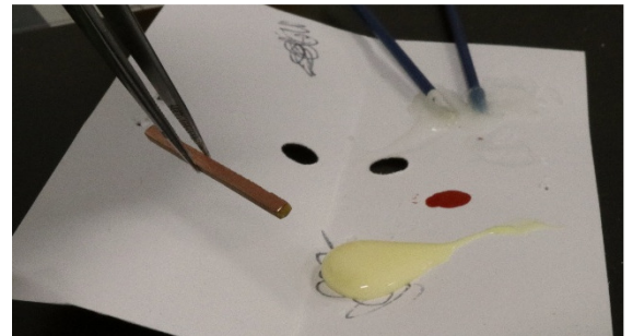
(left) We need to secure the PC ties to the paper template to prevent them shifting during construction, so we use regular carpenters glue to hold them in place.
