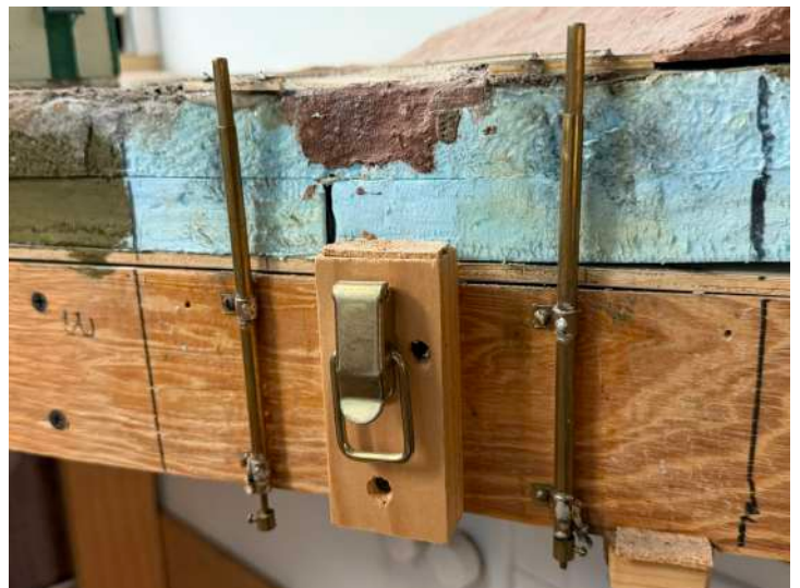
Where the removable section latches to the layout, these two brass tubes serve a dual function. They are spring loaded so they pop up to keep trains from rolling off the end of the track when the removable piece is out. When it's in, they form the contacts for power. There is a similar arrangement for both ends.
