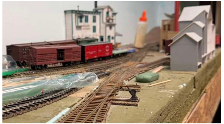
Phil makes his own operating harp switch stands. They sit on top of a small slide switch, which is moved by the switch stand to route power to the frogs. The building mockup in the upper right corner has an cutaway side facing the aisle.
