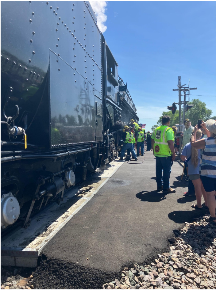
When the Big Boy stopped in Grand Mound, a small army of safety vest-clad workers swarmed it to grease bearings and perform other maintenance tasks.
